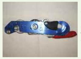
**Petzl stop:** There are a wide range of abseiling devices, which can be used to give the disabled participant as much control as possible during an abseil. A commonly used device is the 'stop' as it is easy to fit to an extension handle. This enables people with very low coordination and strength to control their abseil. Cord can also be attached to the handle to improve grip.
